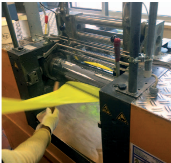
Figure 2 (left): Test of "AG-100 Lemon", 5 % in PVC at 175 °C
